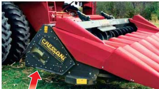
Lateral drive chains lubricated in oil bath.
