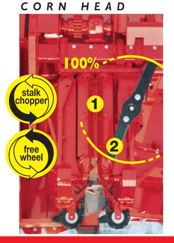
The forward position of the stalk choppers cover **100%** of the rolls' pulling area. This system assures an optimal chop of the stalks in small pieces starting at a minimum safety distance of 3 inches from the ground.
