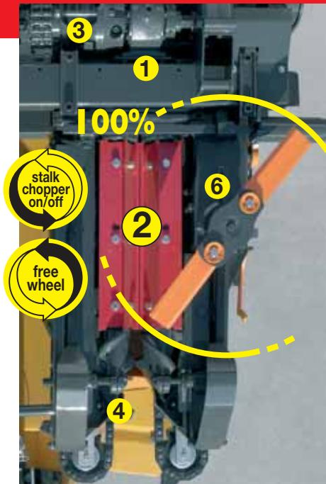
① The ROTO CROSS-CUT and ALUX corn heads are equipped with tempered aluminium alloy gearboxes.
